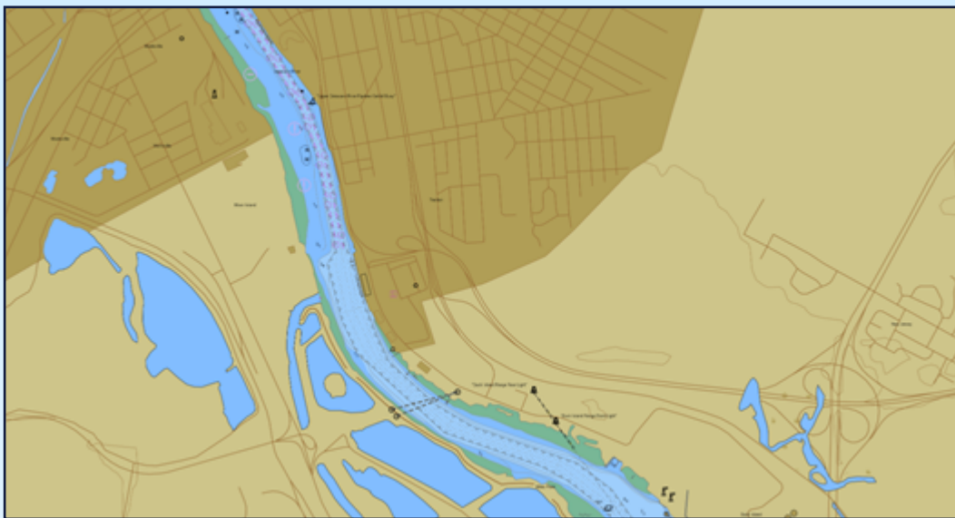
Figure 5. Portion of reschemed ENC Cell US5PHLFJ showing a dark brown urban tint near Trenton, NJ, roads and highways in thick brown lines, and a few topographic contours in thinner brown lines.
